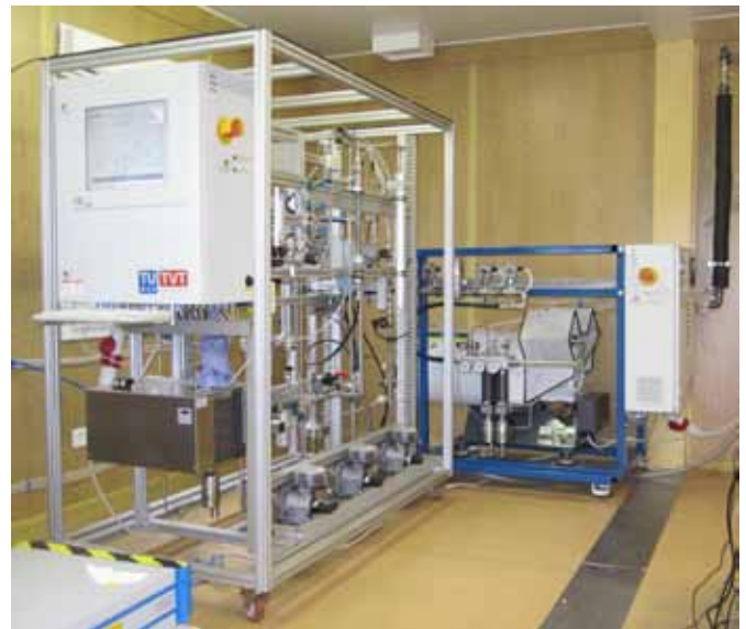
Fig. 3: Membrane tests on hydrogen upgrading at biomass gasification plant in Oberwart
